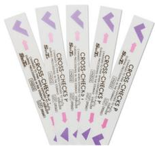
**Chemical indicators** are used every cycle and in each packed item to validate penetration and to ensure vaporized peroxide has made contact with the load.
